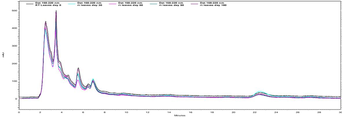
**Figure showing the UV spectra overlay of *A. afra* dried leaves at day 0 and day 180 at site A. ( $\lambda_{\max}$  220nm, retention time 3.52 minutes).**
