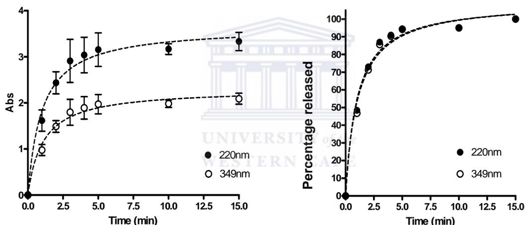
Figure 5.9: The infusion profile (on the left) and percentage release profile (on the right) of the tea bags containing the *A. afra* freeze-dried aqueous extract determined using UV spectroscopy analysis at 220 (-●-) and at 349 (-○-) nm.
