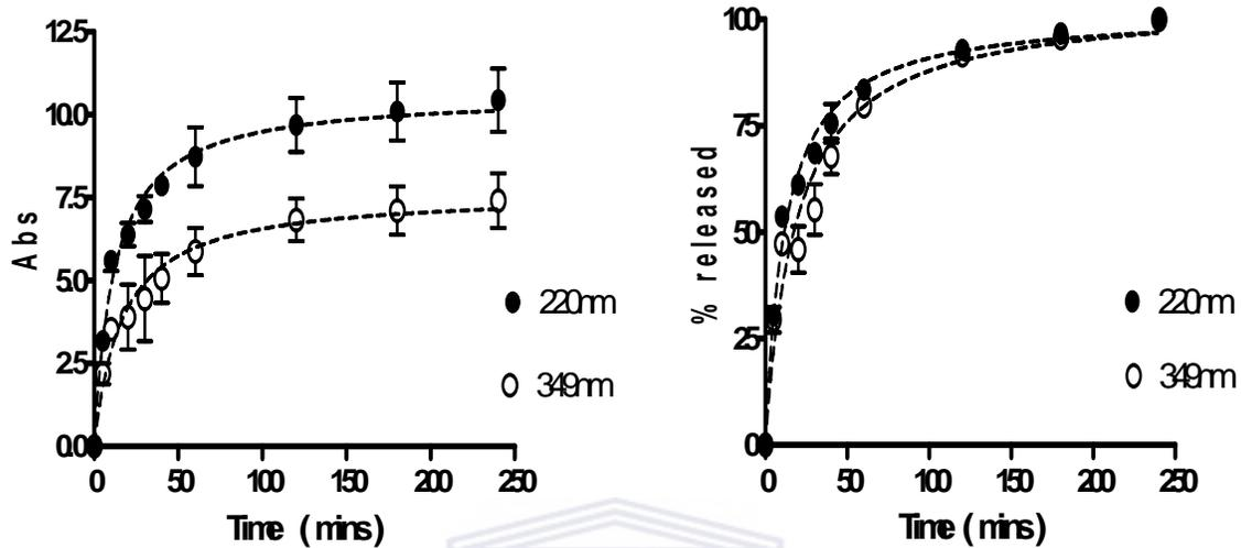
Figure 5.5: The infusion profiles of the *A. afra* loose leaves (on the left) and the percentage release profile (on the right), determined using UV spectroscopic analysis at 220 (●) and 349 (○) nm.
