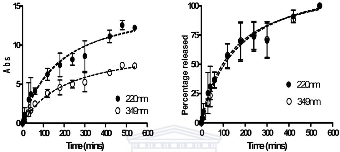
Figure 5.7: The infusion profiles (on the left) and the percentage release profile (on the right) of the tea bags containing the *A. afra* leaves determined using UV spectroscopic analysis at 220 (-●-) and 349 (-○-) nm.
