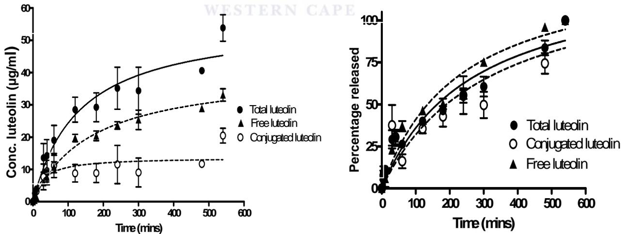
Figure 5.8: The infusion profile of luteolin (total -●-, conjugated -○- and free -▲-) release (on the left) and the percentage release profile of luteolin (on the right) from the tea bags containing the *A. afra* leaves.
