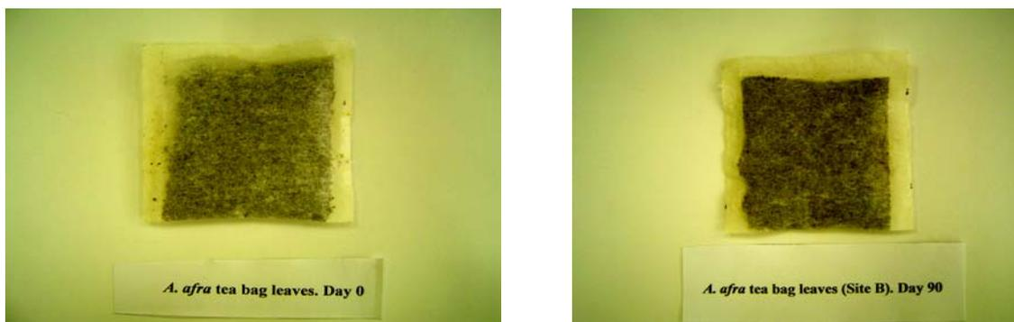
**Figure 5.12:** Shows, on the left, a tea bag containing the *A. afra* leaves at day 0 and on the right, a tea bag containing the *A. afra* leaves after 90 days storage at conditions of 40°C /75% relative humidity. Note the green colouration on the tea bag surface after 90 days.
