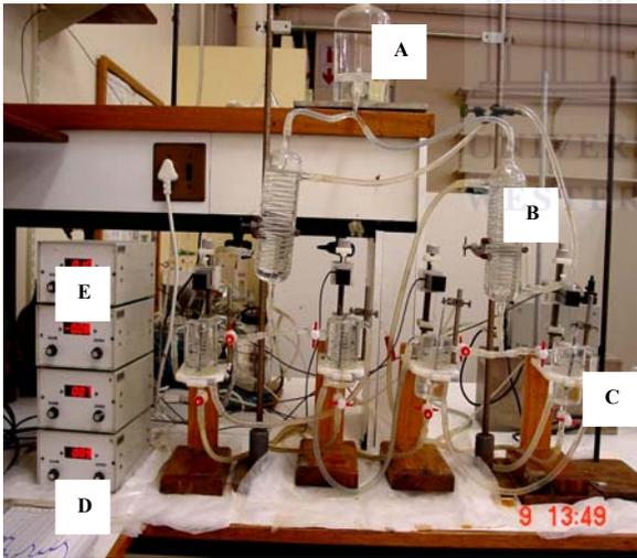
**Figure 5.2** The organ bath system used for evaluation of the activity of the plant materials. A is the bath reservoir containing Krebs Henseleit solution, B is one of the water-jacketed glass reservoirs C is the water bath temperature controller, D is the 4-pen strip chart recorder and E is the signal amplifiers.
