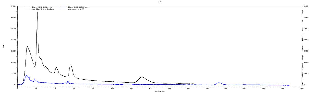
Figure showing the UV spectra overlay of *A. afra* freeze-dried aqueous extract in tea bag at the beginning and end of stability testing at site A. ( $\lambda_{max}$  220nm, retention time 3.52 minutes).
