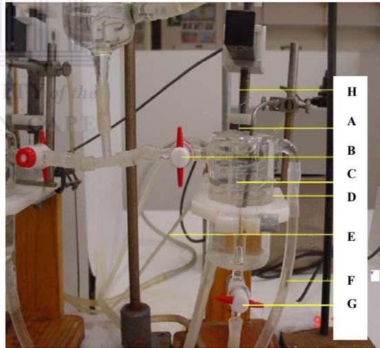
**Figure 5.3:** A close up picture of a single organ bath. A shows cotton thread used to tie the tissue to the transducer, B is the Krebs' inlet tap, C shows the suspended tissue, D shows the bath, E shows the gas inlet, F, shows one of the pipes to the water-bath that transport warm water to maintain the temperature, G shows the Krebs' outlet tap and H shows the transducer.
