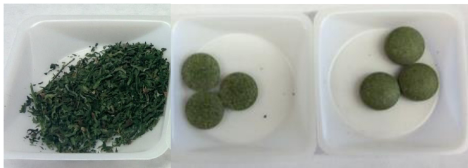
Fig. 2. Three granulation sizes of A. annua leaves; two were pressed into tablets. Granulation size L to R: 2.0 mm (could not form into tablets), 0.6 mm into tablets, ~100–150 \mu\text{m} into tablets. Tablet weights are ~0.17 and ~0.30 g, respectively; tablet dimensions were 10 mm diameter, 3 mm maximum depth.
