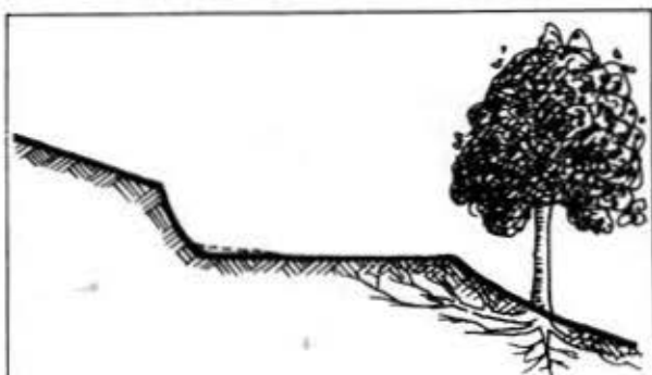
FIGURE 9.12 BENCHES CUT INTO HILLSIDES ON CONTOUR
